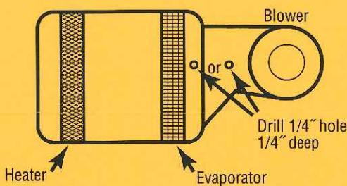
4. In the neck area between the blower and the evaporator drill a 1/4" diameter hole as close to the evaporator as possible. The hole should be located in an out-of-the-way place and can be located on the top, side or bottom areas.
