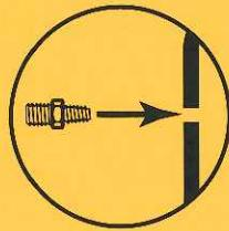
5. Use a 3/8" wrench to install insert adaptor into the hole in the plastic. The adaptor is self-tapping and should thread in easily.
