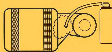
8. Allow A/C system to run for one minute, then shut down engine to allow evaporator to soak in the foamy cleaner. At this time remove the can hose from the threaded adaptor and either:
