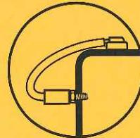
9. Allow vehicle to sit for 10 minutes then start again making sure A/C is on Max and blower is at highest setting. After about 8 minutes of running and with the A/C system still on, install BG Frigi-Fresh® into the fresh air vents on the outside of the vehicle.
