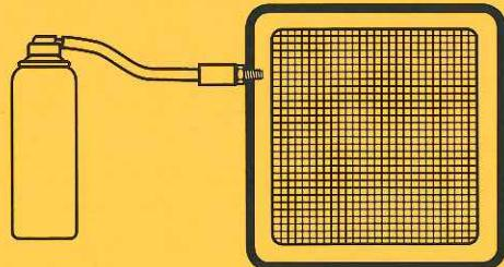
6. **Shake can** of BG Frigi-Clean® vigorously before using. Connect hose from the can to the threaded adaptor.
